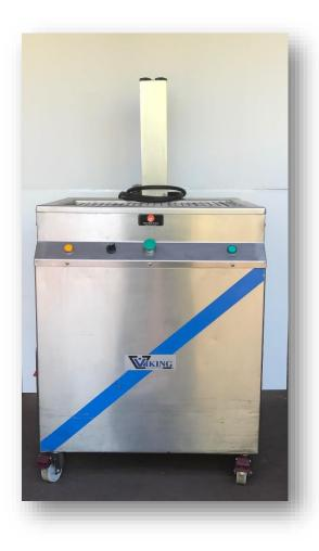
This original style BMSS dip tank has had the motor replaced as well as the bearings for the lifting basket. An added bonus is an additional time delay.
